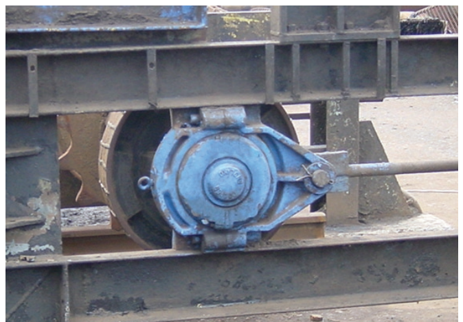
A tension take-up unit with blanking plate on a sugar mill conveyor
